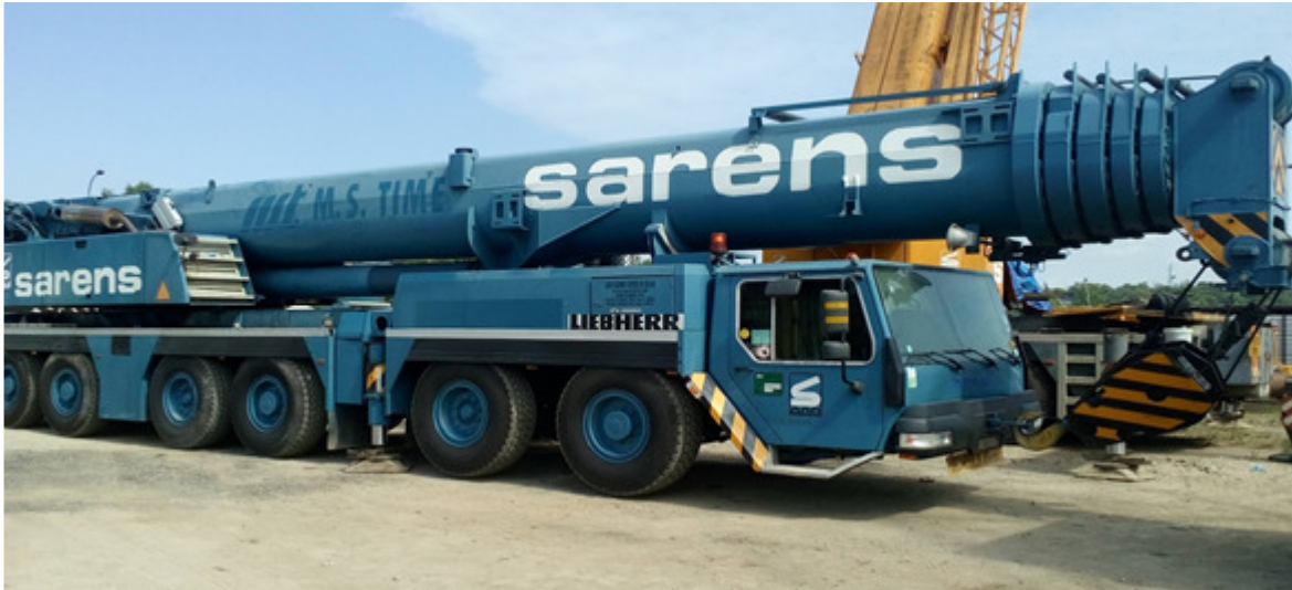
Equipment: LIEBHERR LTM1250-1 (4127) LOCATION: Malaysia
