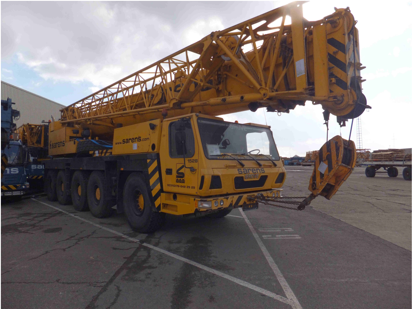
Equipment: Grove GMK 5130-1 (1528) LOCATION: Europe
