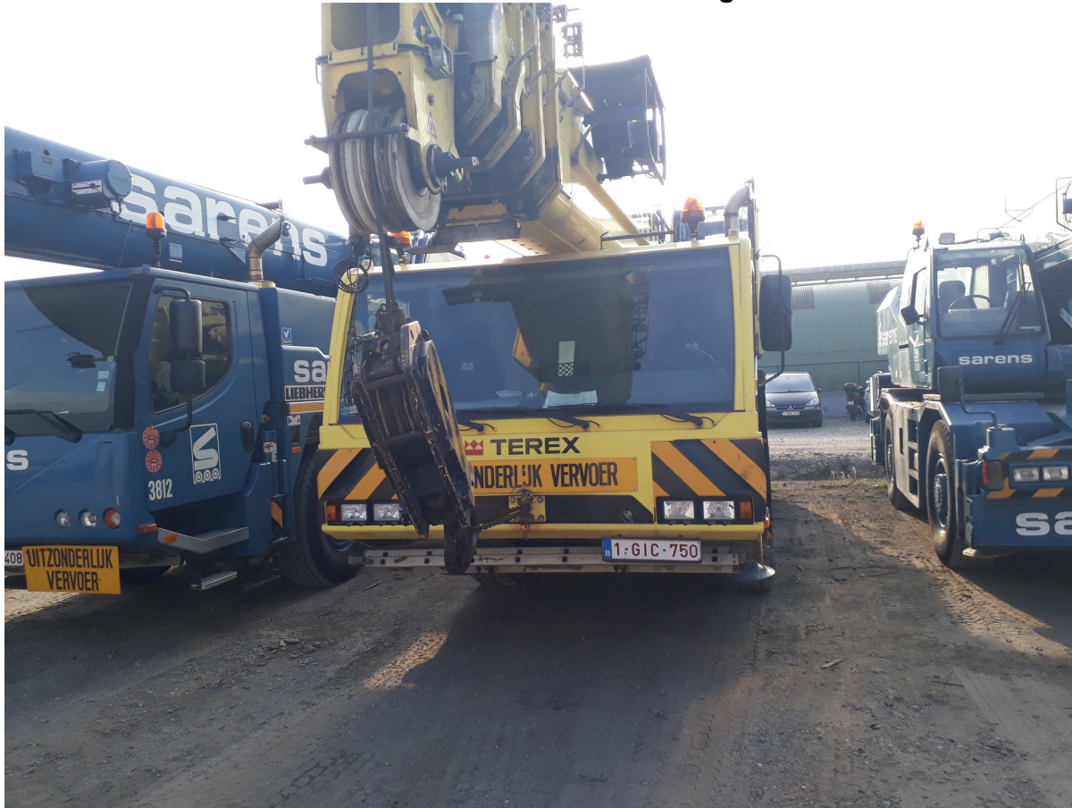
Equipment: Terex-Demag AC50-1 (5034) LOCATION: Belgium
