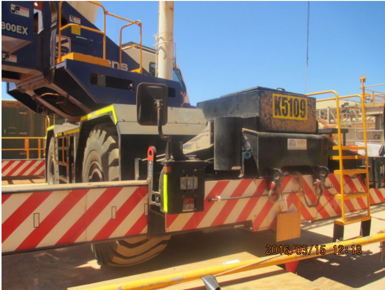
Equipment: TADANO GR800EX-2 (5109) LOCATION: WA, AUSTRALIA
